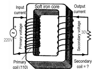
What is electromagnetic induction? What type of transformer is given in the diagram? Calculate the number of turns in secondary coil.  $1+0.5+2 = 3.5$
